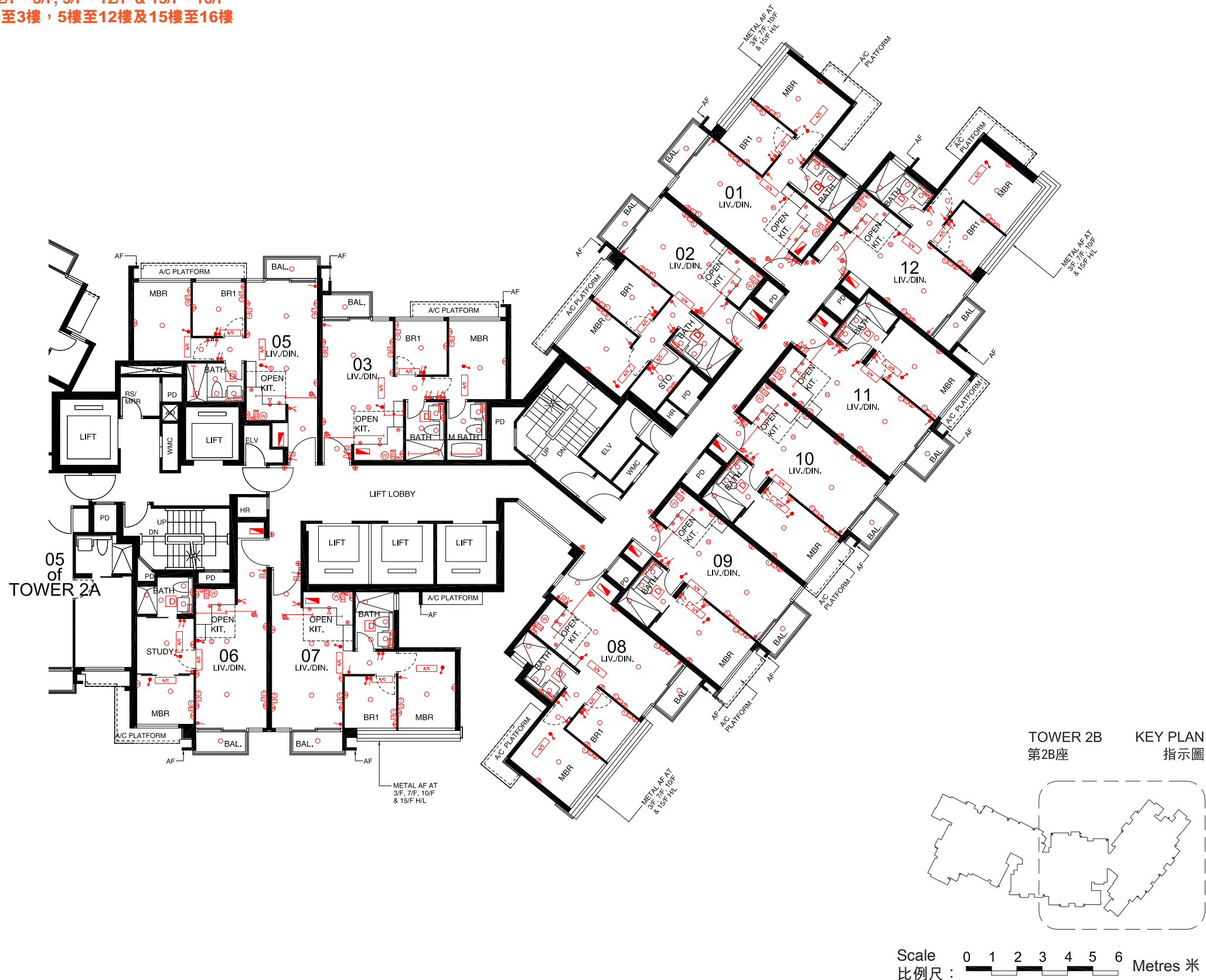
Mechanical and Electrical Provisions 機電裝置說明表
